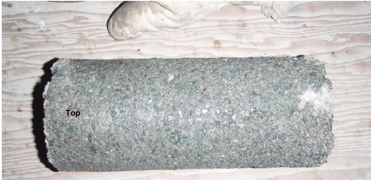
Photo 12 : Close up of drilled core 67, drilled around station 0+84 around the centerline.
