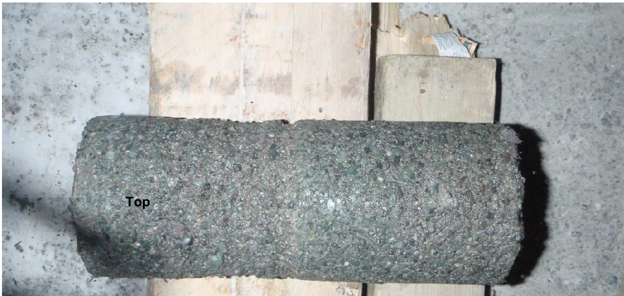
Photo 11 : Close up of drilled core 66, drilled around station 1+11 on the upstream. Note that less glycol was used when drilling the first half of this core.
